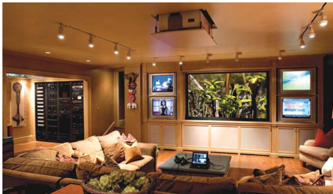
The client's former media room, showing Runco VX-5000c on Display Devices lift with 107" Stewart motorized screen, flanked retracting 32" Sony CRT televisions. The base cabinets concealed a JBL Synthesis 2 system, which was run from the series of racks at the left. The house-wide AMX automation system was run from there as well.
